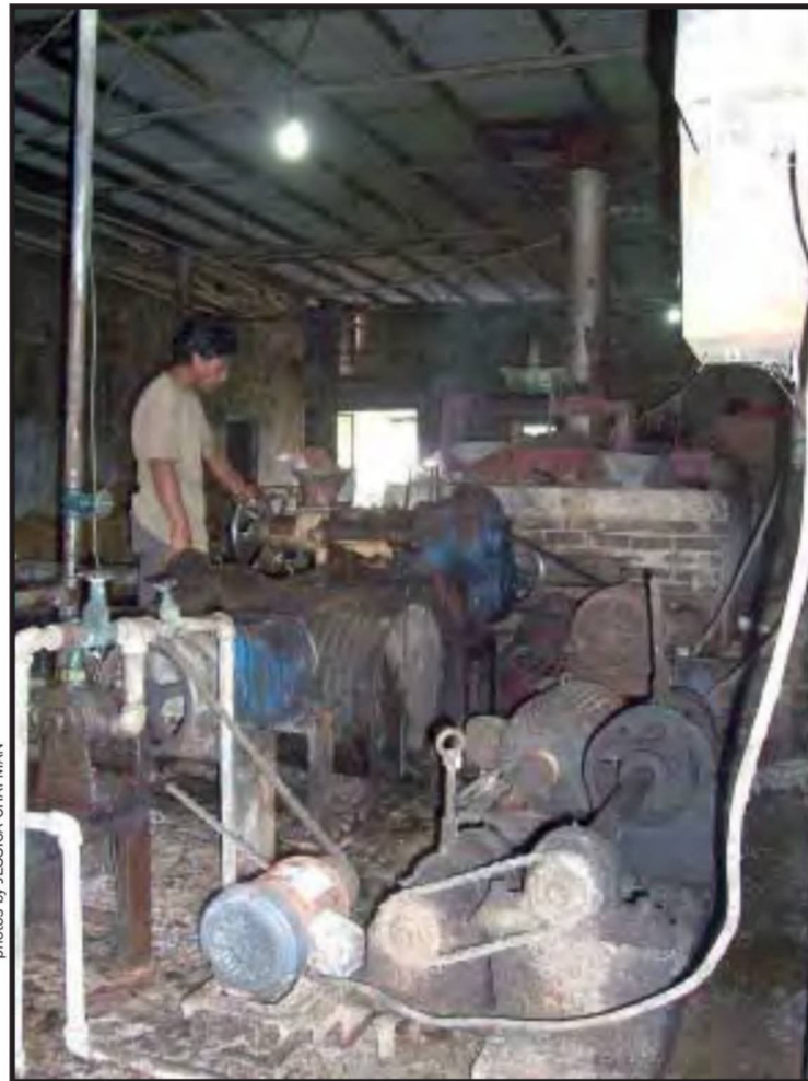
PCP employee John Peter tends to an expeller, which extracts oil from heated copra. The oil is then directed to a filter press where it is refined even further.
