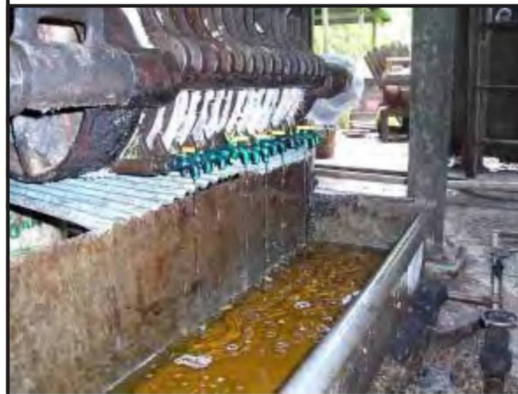
Coconut oil drips from a filter press used to extract any remaining impurities from the processed oil. From here, it will be transported to storage tanks where it awaits purchase. PCP is able to produce 150 gallons of coconut oil in one day.
