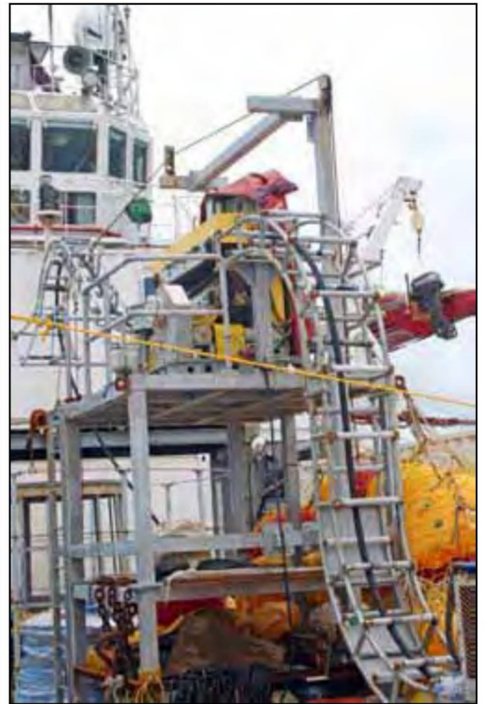
Fiber optic cable on the Amarco Cheetah ready to be run in Pohnpei's Lagoon
