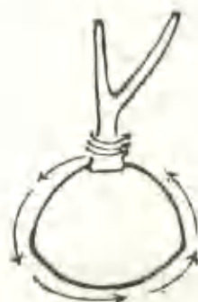
Figure 13—Method of securing outrigger attachment to float. The arrows indicate lashing
