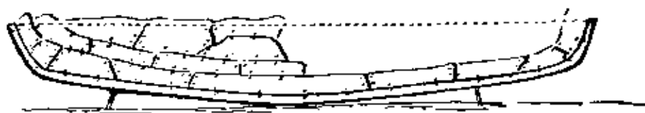
Figure 7—Hull in process of construction. Note how tiers of planks follow curve of the stem. The dotted line is gunwale level
