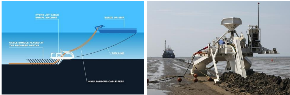
Figure 1. An example of submarine cable ploughs at sea and being towed from shore to deeper water by a cable laying ship
