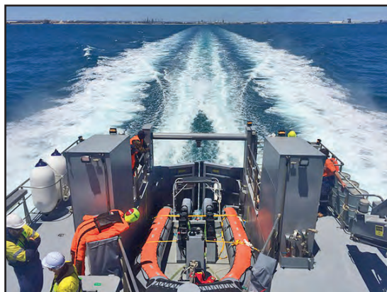
Guardian Class vessels have a stern launch capability for the embarked Rigid Inflatable Boats
