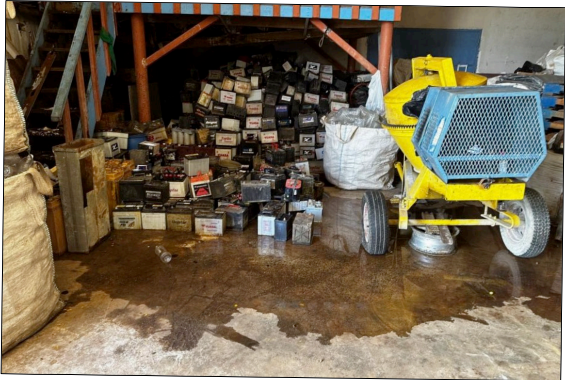
Photo 15: Overview of a lead-acid battery pile located inside the Recycling Center observed sitting on a large puddle of rainwater. Approximately 200–300 batteries were estimated. Photo taken standing on top of floor drain.
