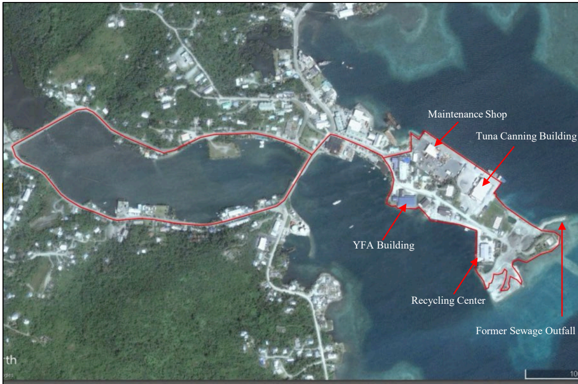
Photo 2: 2005 – Subject property, Colonia. The subject property appears fully developed. The wharf inside the gated area has been filled. The maintenance shop, YFA building, recycling center and tuna canning building are denoted by the red arrows. The majority of the former sewage outfall is now underwater.
