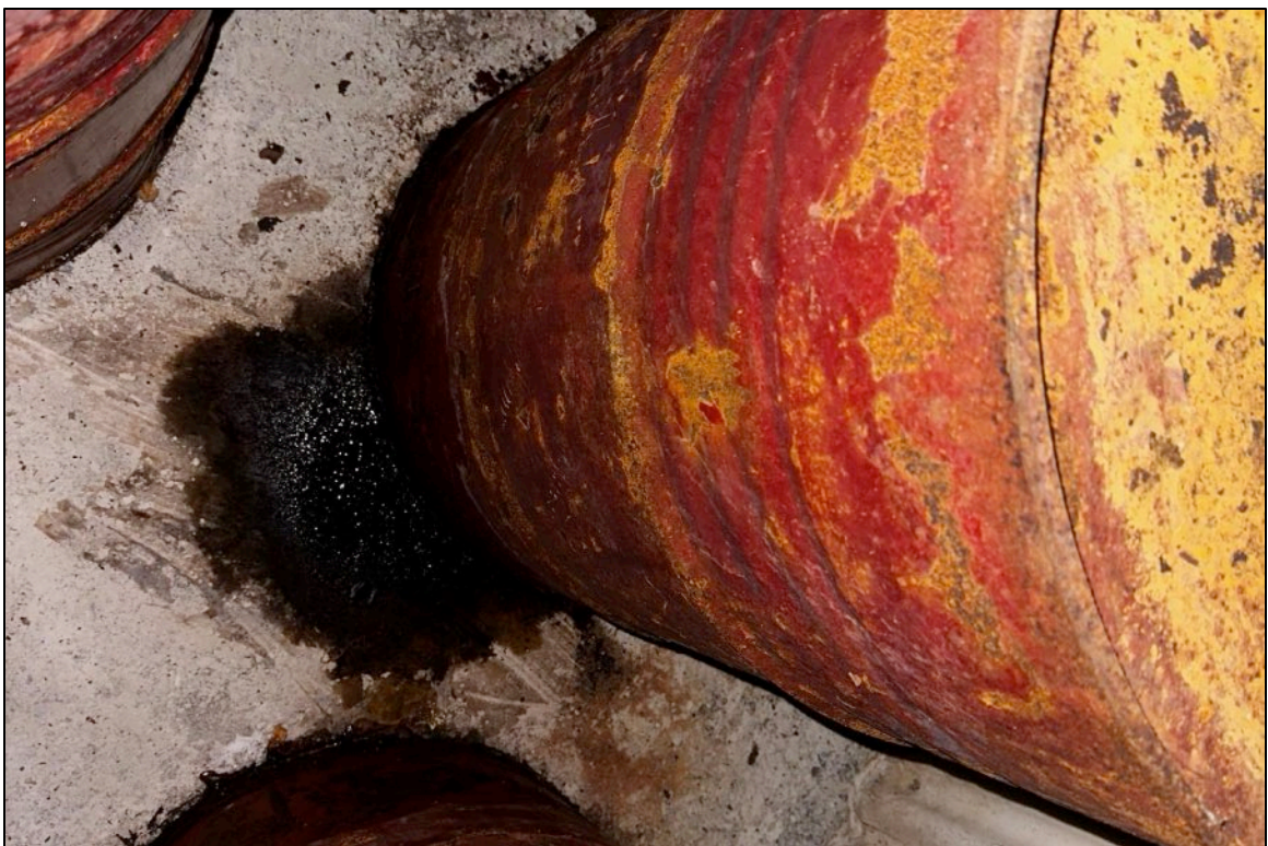
Photo 2: Close-up view of one of the drums leaking de minimis amounts of oily substance on the concrete floor.
