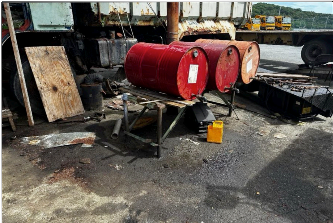
Photo 6: Closer look at three 55-gallon drums containing hydraulic oil. Note: Extensive staining observed on the concrete surface. This type of staining was observed throughout the premises. Photo is looking north.
