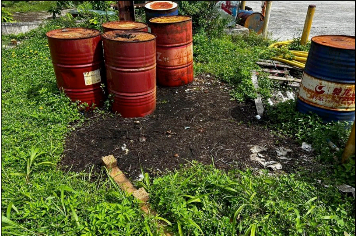
Photo 3: Four empty 55-gallon metal drums observed near the northeastern corner of the former tuna canning facility. Note stressed vegetation surrounding the drums. Photo is looking northwest.
