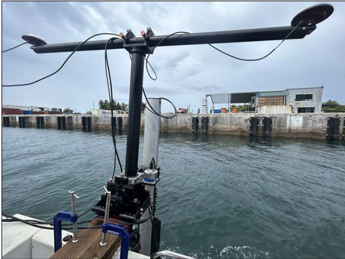
Figure 2-7. Final multibeam sonar system setup on the survey vessel
