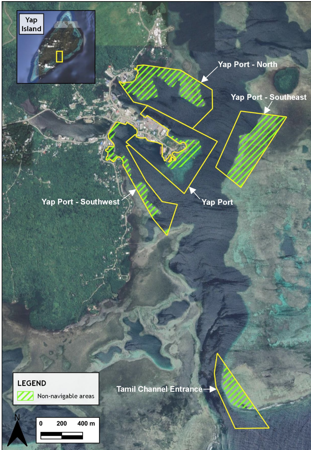
Figure 2-12. Yap Port and Tamil Channel Entrance areas investigated during side-scan and magnetometer surveys outlined in yellow Non-navigable survey areas are shown in green
