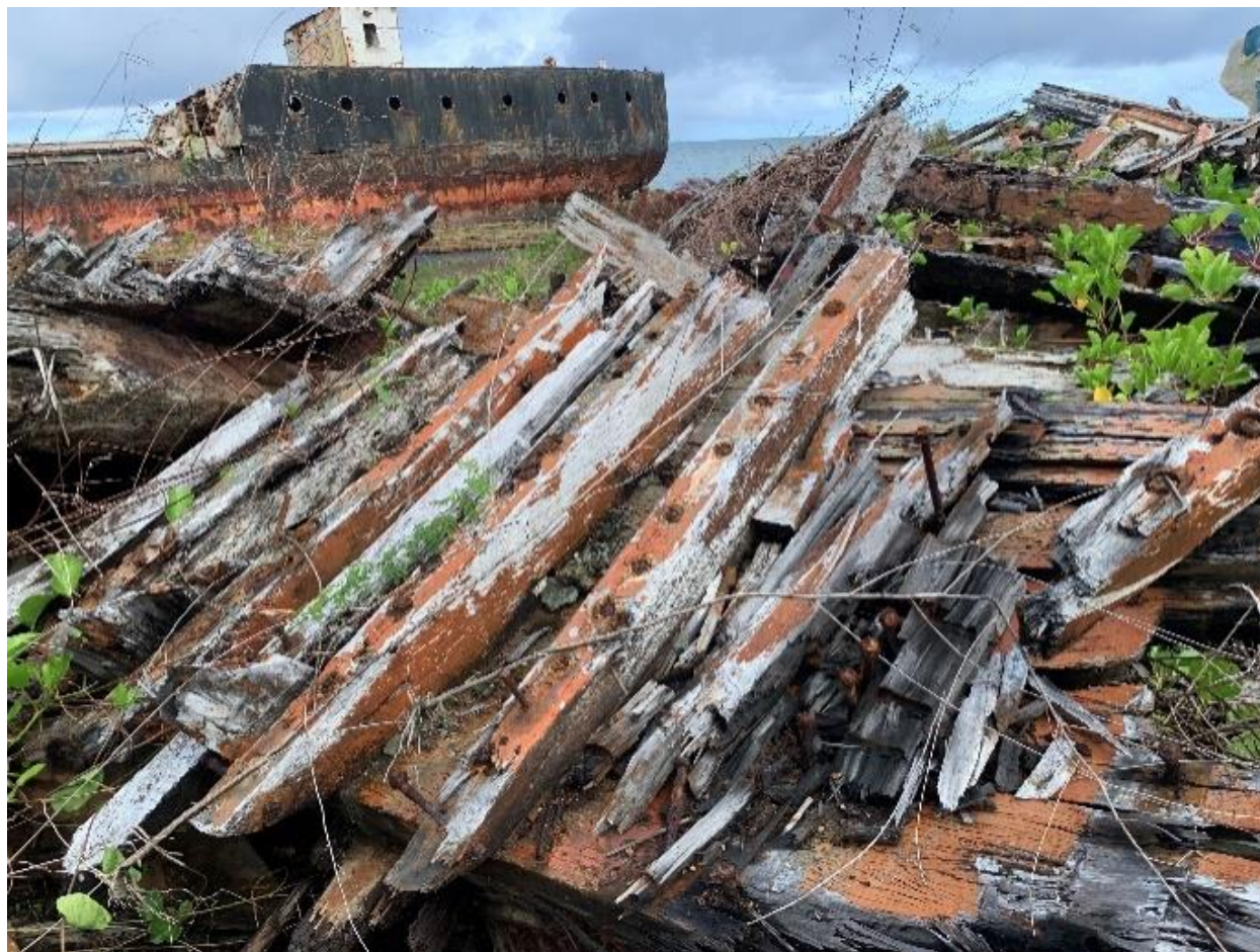
Figure 3-77 Frames and Outer Hull Planking (Photo by AECOM)
