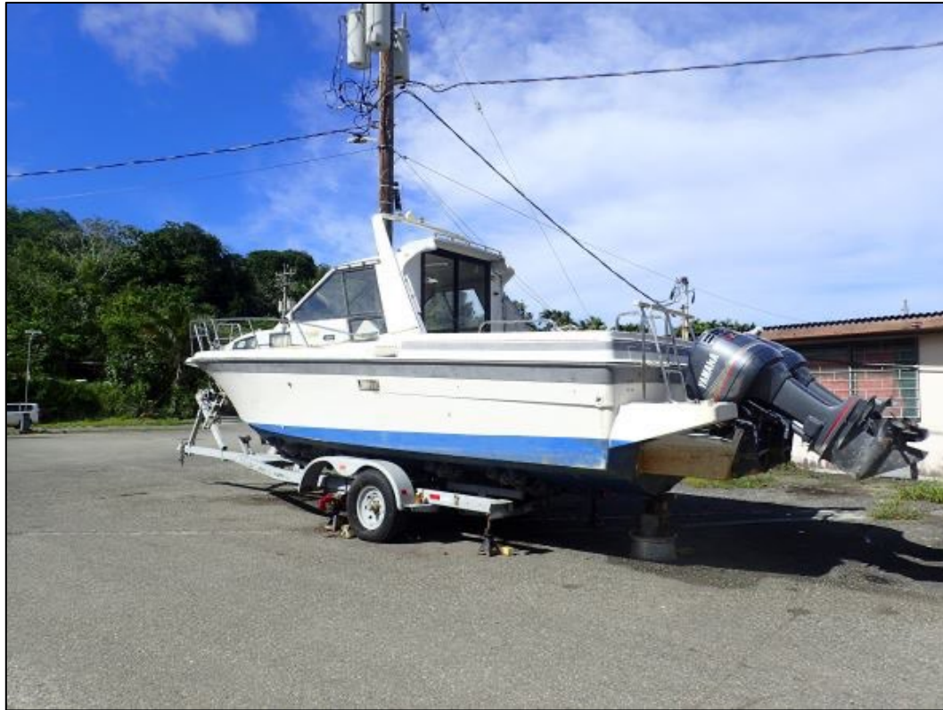
Figure 2-4. Survey vessel used for side-scan, magnetometer, multibeam sonar, and drop camera surveys
