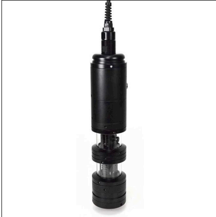
Figure 2-16. SideWinder 360 camera used to investigate channel markers and other areas of interest in Tamil Channel (Splashcam, 2018)
