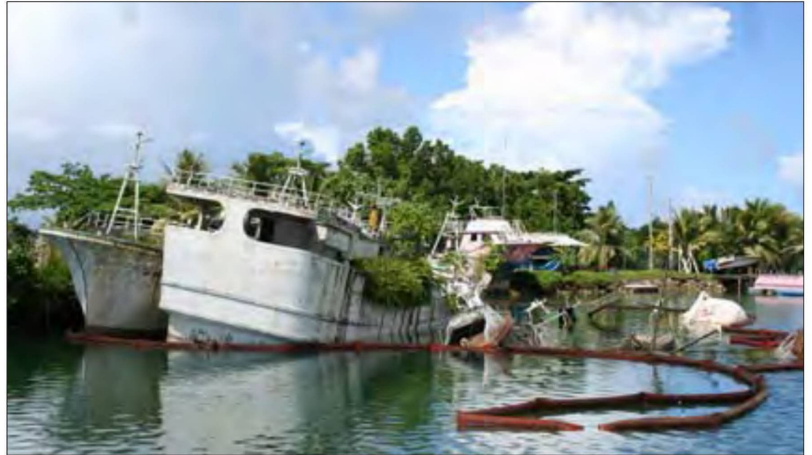
EDA fishing vessels sinking off Deketik in Pohnpei. Fuel barricades seem to have been permanently placed in order to keep fuel from the vessels from further contaminating the harbor. The place reeks of diesel fuel.
