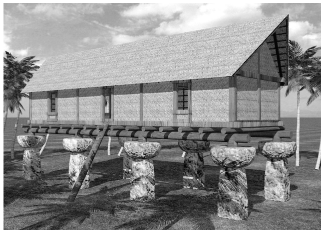
Fig. 7: Architectural engineering reconstruction of a latte house structure in the Mariana Islands. Original graphic prepared by John Aguon, reproduced by permission from Laguana et al. (2012).
